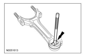
2. Measure the telescoping gauge with a micrometer. Verify the diameter is within specification.
